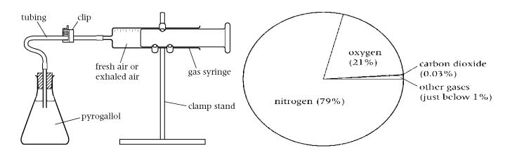
The gas syringe was filled with 100 cm<sup>3</sup> of air. Pyrogallol absorbs oxygen. The apparatus was left for 20 minutes.
