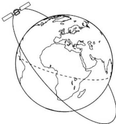
*When the satellite reaches this point on its next orbit, the Earth will have spun round and a different part of the Earth will be under it.*
